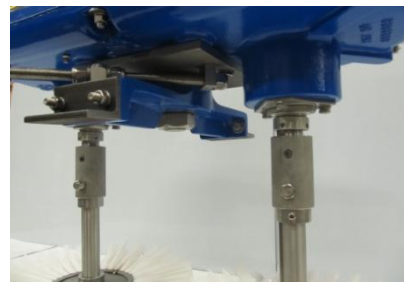
Split Shaft allows one-bolt removal of brush assembly
